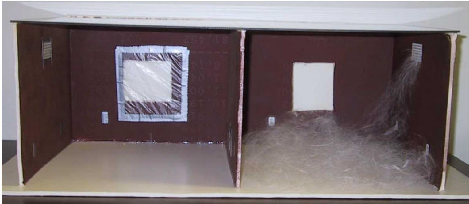
One of two scale models demonstrating a room prepared for Sheltering-In-Place versus a room that has not been prepared. The room on the right demonstrates a chemical vapor entering through the building's ventilation system, windows and electrical outlets.
